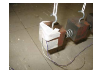
Piezoelectric accelerometer attached to last block
